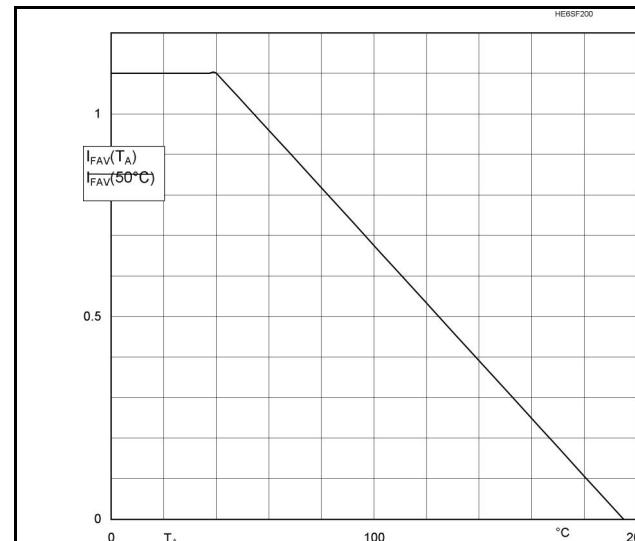
Fig. 2 Rated forward current vs. ambient temperature <sup>1)</sup>
