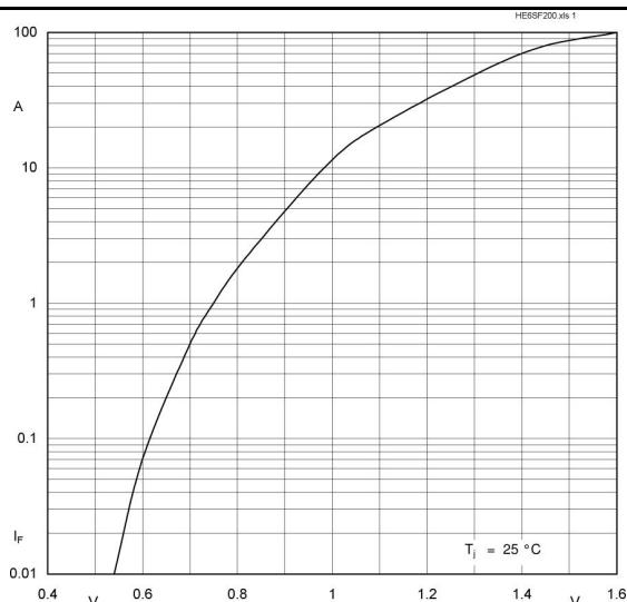
Fig. 1 Forward characteristic ( typical values )
